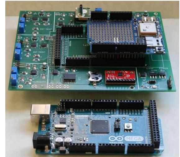
The Arduino Mega, custom MegaSat board, and Adafruit GPS logger is used as the LaACES payload core
