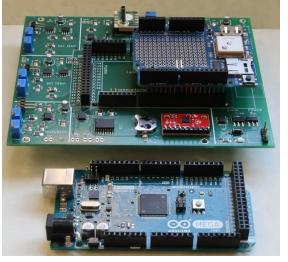
The Arduino Mega, custom MegaSat board, and Adafruit GPS logger is used as the LaACES payload core
