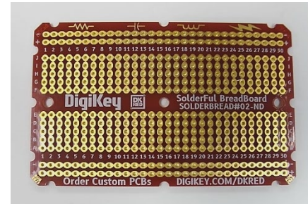
Figure 11: PCB breadboard. Notice this PCB has the same layout as the breadboard. The columns and rows are numbered differently.
