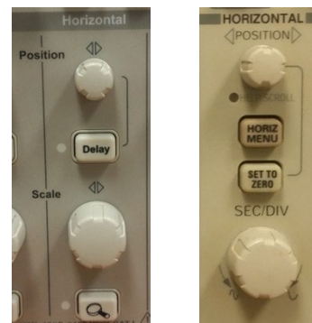
Figure 7: Horizontal controls. Since the scale is shared there will usually only be a single set of these.
