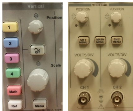
Figure 6: Vertical Scale Controls, the left image shows a shared control used by 4 channels, selected via the channel button. The right image has individual controls for each channel.
