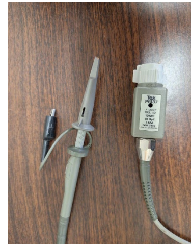
Figure 2: Oscilloscope probe, which has 10x attenuation, 10 MOhm impedance, and 10.8 pF capacitance.
