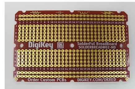
Figure 13: PCB breadboard. Notice this PCB has the same layout as the breadboard. The columns and rows are numbered differently.
