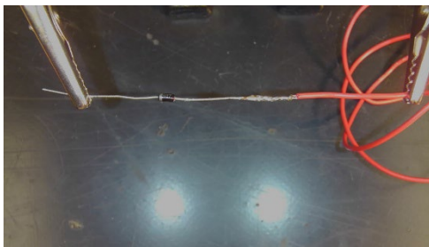
Figure 4: Soldering a red wire to the diode lead. Notice we have soldered this to (+) lead. We will not be able to see the stripe on the diode once we cover it with waterproofing
