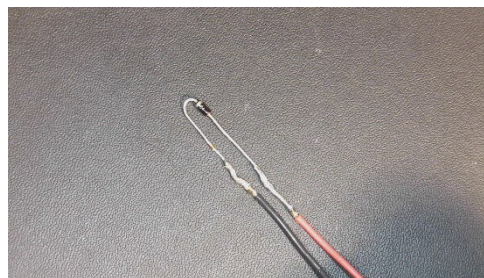
Figure 3: Diode with wires soldered to both leads
