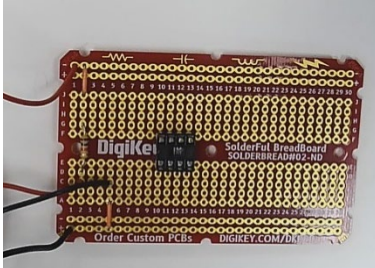
Figure 24: Soldering Op Amp socket in the PCB
