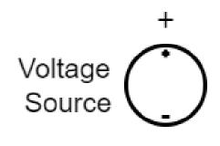
Voltage sources usually increase the voltage, so choosing the negative terminal as 0 you would measure an increase in voltage at the positive terminal
