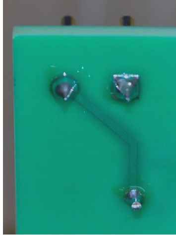
Figure 22: Backside of J1 with a single pin soldered.
