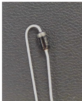
Figure 109: Pre-bent diode for temperature sensor.
