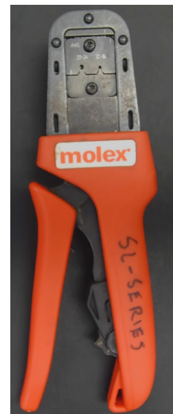
Figure 110: The crimps used for connecting sensors. Middle shows the approximate length of wire you should strip for crimping, notice the back set of tabs on the crimp should fold over insulation and the right front on bare wire. Right: shows the crimping tool.
