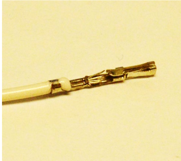
Figure 111: Wire lead after crimping. Again, notice the back set of tabs on the crimp should fold over insulation and the right front on bare wire
