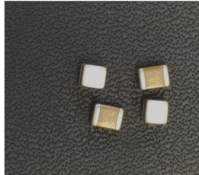
Figure 91: Four 10 uF capacitors.
