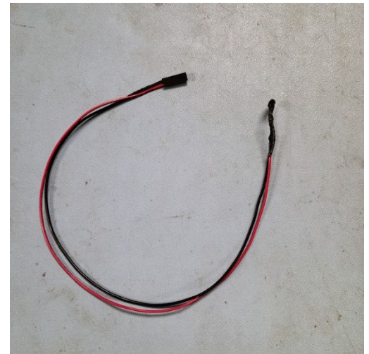
Figure 1 Soldered and insulated diode for temperature sensor. Note bare wire ends may be used instead of crimped connection
