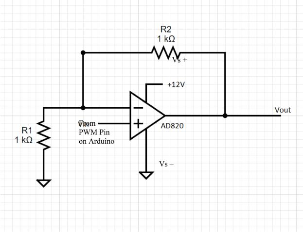
9) Measure the signal at the output of the amplifier. If possible, monitor the input voltage on 1 channel and the output voltage on a second channel at the same time. How do they compare?
