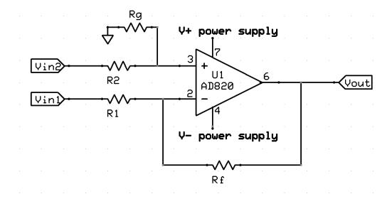
A difference op amp has an input into both the negative and positive terminals.
