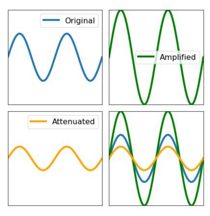
When a signal is too small to be measured correctly, the signal can be amplified. **Amplification** is the process of increasing the amplitude of an electrical signal. (Gain >1)
