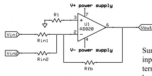
Summing op amps have multiple inputs are connected into a single terminal. Can be inverting (shown here) or noninverting.
