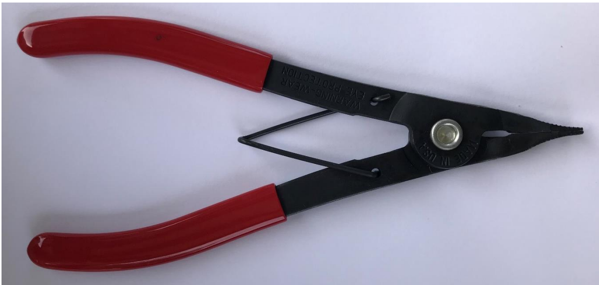
Figure 3: This is the tool you will use to unstack the Shield and the Mega. Using this lock ring spreader pliers will help prevent pins from being bent.
