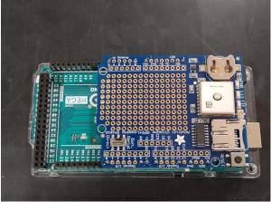
8. After we soldered a couple pins of each header we can remove the shield from the Arduino. To prevent bending the pins use the ring pliers to push the shield and Arduino apart from both sides of the shield. After we remove be sure to check that all of pins are still in place.
