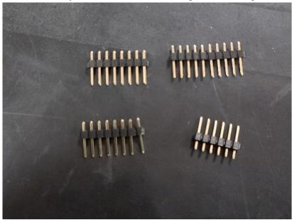
5. We are going to use the Arduino to hold the pins while we are soldering them to the shield. Install the pins long side down into the Arduino with the short side sticking up. Install the header as shown in the table below:
