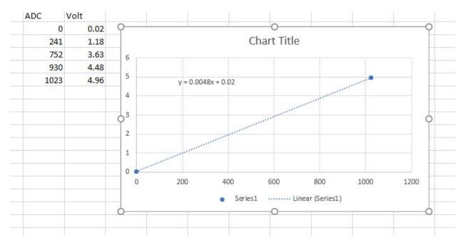
12. Write a function in your code that takes ADC value read and calculated the corresponding voltage using the equation you just determined. Note because we want the voltage, slope and intercept to be decimals we should declare them as floats
