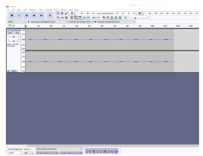
Using the select tool (the one that looks like an I) we can highlight a single beep in the timeline. We want to then select "Plot Frequency" from the Analyze menu. After doing so we should see histogram of various frequencies on the X axis with decibels (dB) on the Y axis.
