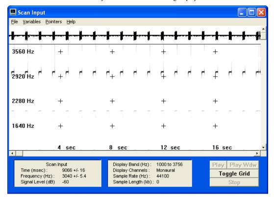
As you move the cursor around the screen notice how the box in the lower left shows you the time, frequency, and amplitude of the recorded signal. This is the tool you need to make meaningful measurements with *SkeeterSat*. *Spectrogram* has many other features and capabilities. Spend some time reading through the HELP file within the program.
