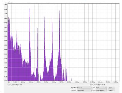
analyzes the sound, and we should just leave them on the default values of "Spectrum" and "Rectangular Window". The axis box lets us switch between a linear and log scale for the frequency axis, we want linear. The size drop down lets us select the number of frequency bins the data is broken into. So, I higher size number means we will have better resolution but if we set it too high we might not be able to see the peaks,
