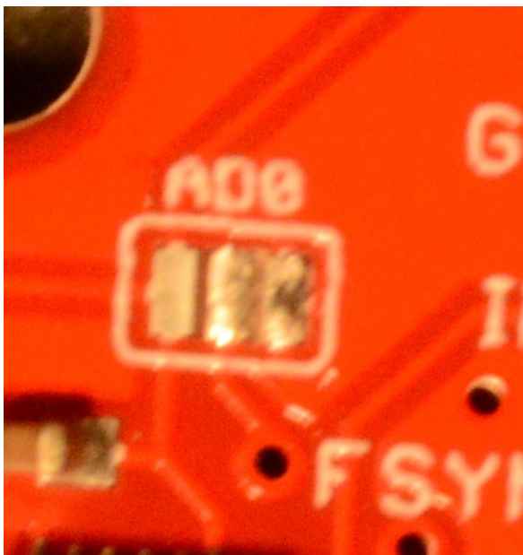
Figure 85: Address jumper AD0 after the connection between center and right pads has been removed.
