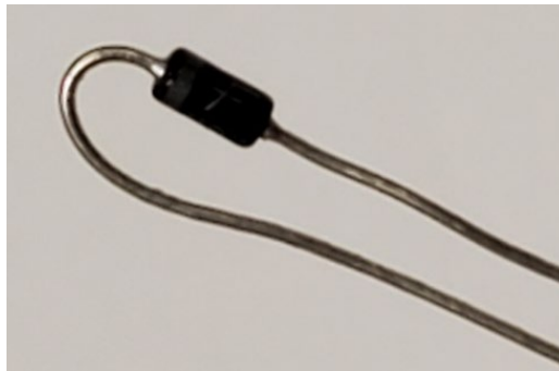
Figure 101: Pre-bent diode for temperature sensor.
