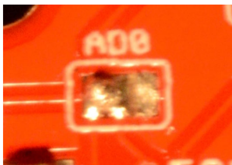
Figure 84: AD0 jumper after the connection has been made between the left and center pins. In this configuration the I2C address will be 0x69.
