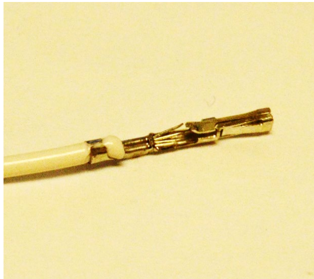
Figure 102: Wire lead after crimping.
