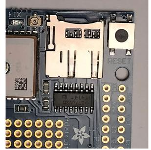
The Adafruit Ultimate GPS Logger Shield's microSD socket. It is next to the Reset button. When inserting a microSD card, it will latch once fully inserted. To eject simply push the card in again
