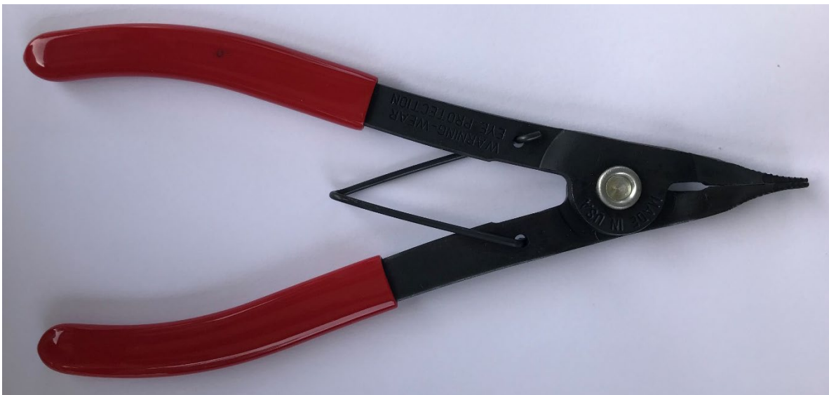
Figure 3: This is the tool you will use to destack the Shield and the Mega. Using this lock ring spreader pliers will help prevent pins from being bent.
