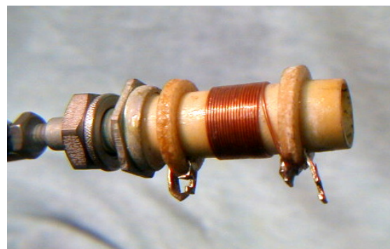
Adjustable air-wound inductor
