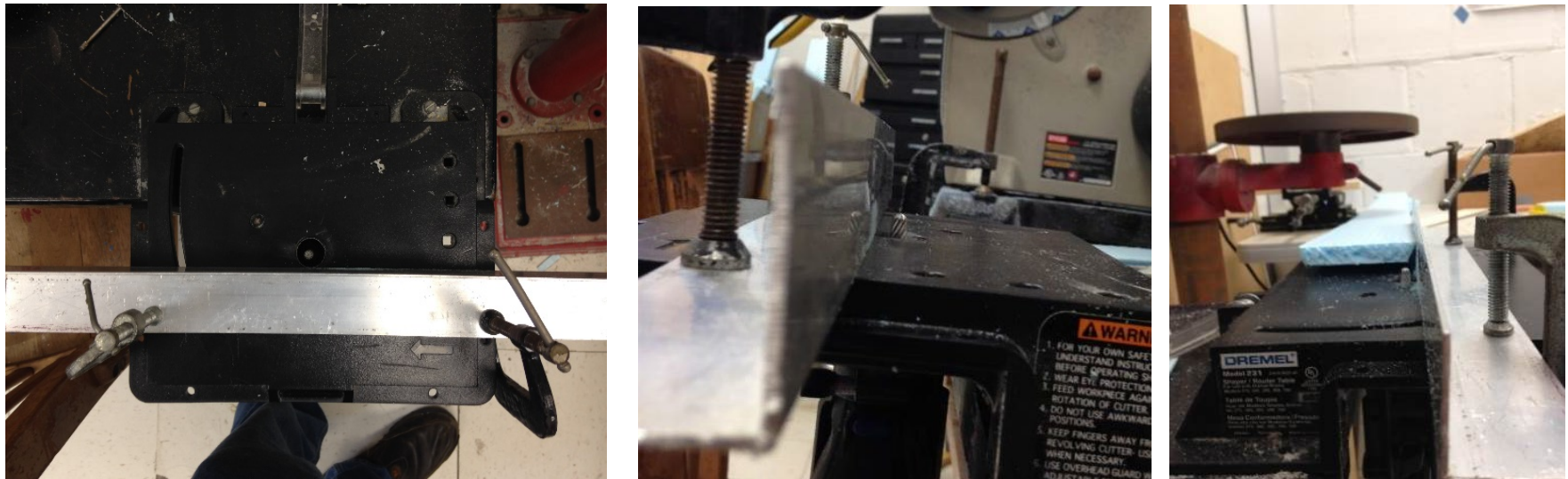
Figure 5: Setting up the Dremel tool and making grooves for the straws
