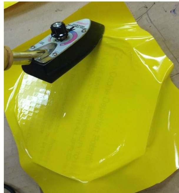
Figure 9: Applying econokote to the endcap
