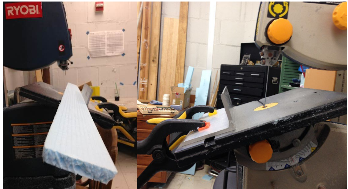
Figure 4: Bandsaw table angled at 22.5^\circ for the wall cuts
