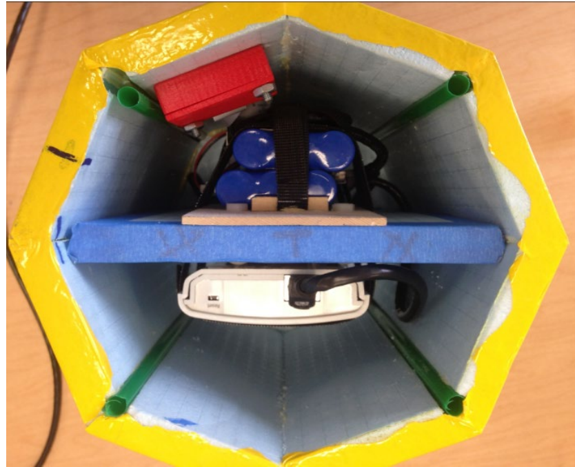
Figure 10: An top-view of an old LaACES video payload with foam inserts and mountings
