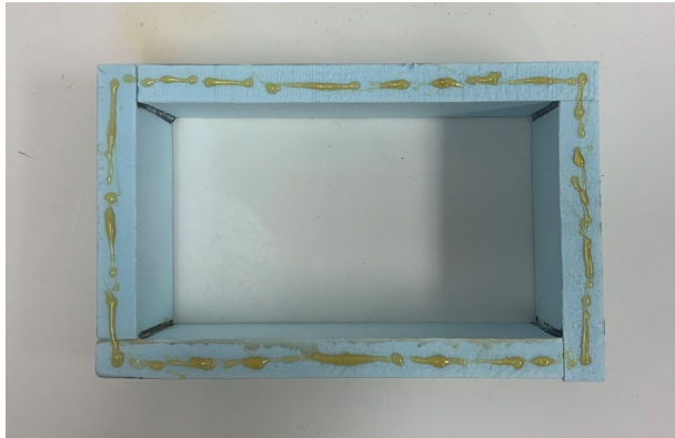
Figure 15: Apply glue to the bottom edge of the inner wall piece
