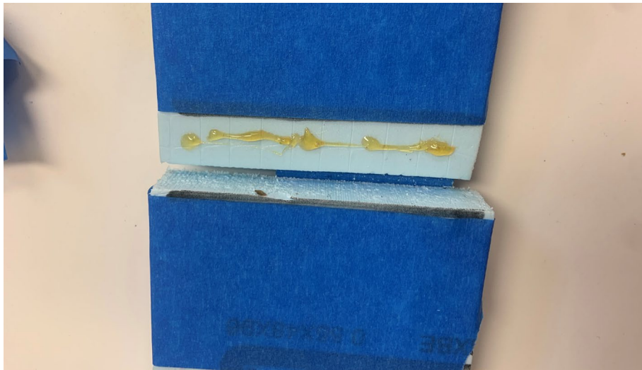
Figure 7: Apply Polyurethane glue to the right side of the joint
