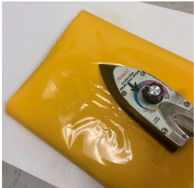
Figure 23: Start in the center and work your way out
