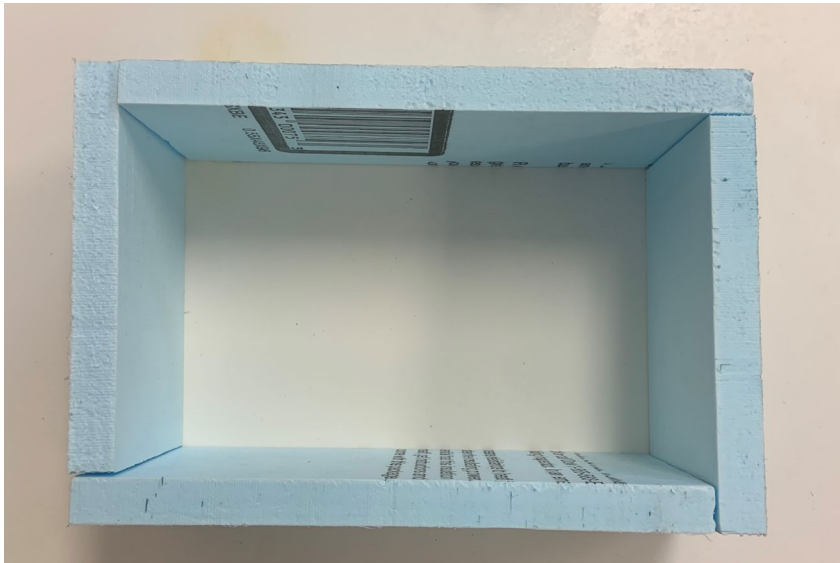
Figure 3: Arrange the walls to ensure they're flush
