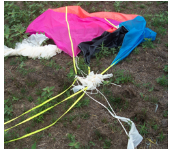
The ACES01 parachute shrouds tangled with balloon remnants
