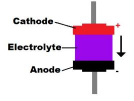
**Electrolyte** – Chemical solution or substance that creates chemical reactions to create the battery voltage difference
