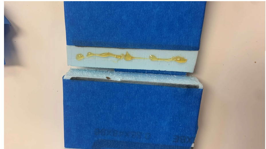
Apply tape to both sides of the joint before gluing
