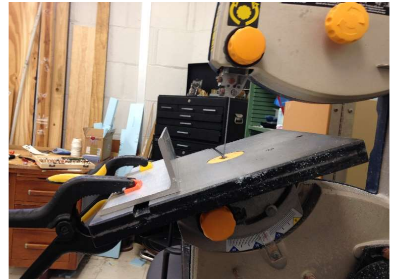
A bandsaw with table angled down
