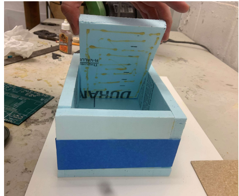
Figure 13: Place the inner bottom piece on the outer bottom piece
