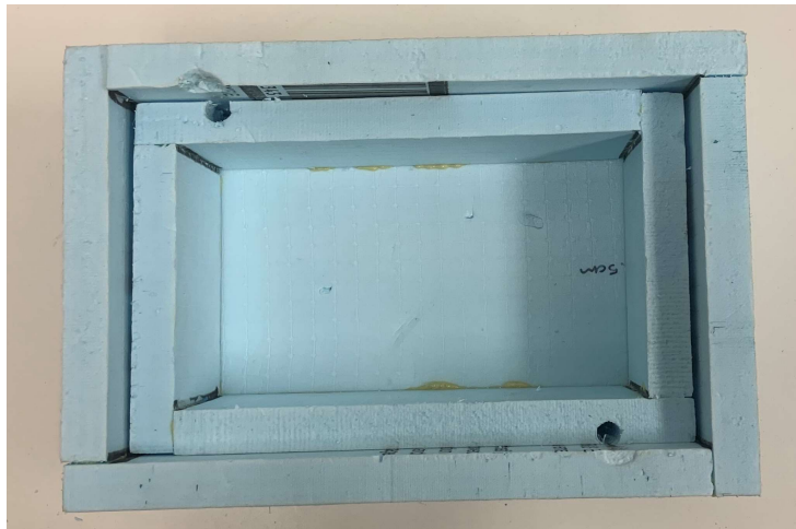
Figure 18: Make holes in the inner wall for the straws
