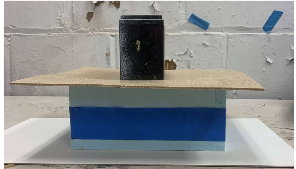
Figure 14: Apply pressure as the glue cures with weights
