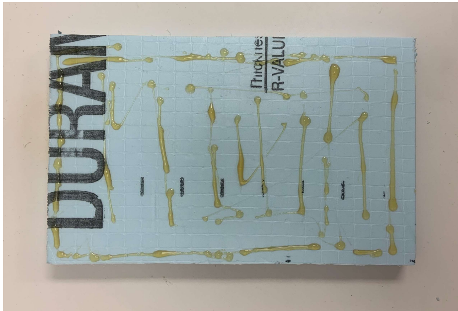
Figure 12: Apply glue to the bottom side of the inner bottom piece
