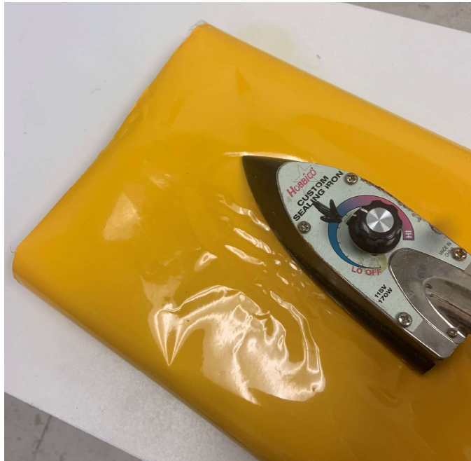
Figure 23: Start in the center and work your way out
