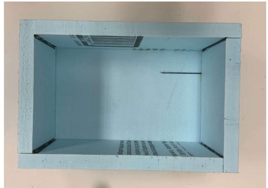
Figure 11: Set the outside wall piece on the outer bottom piece
