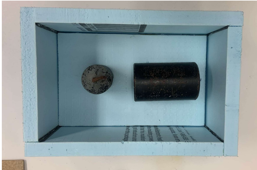
Figure 14: Apply pressure as the glue cures with weights
