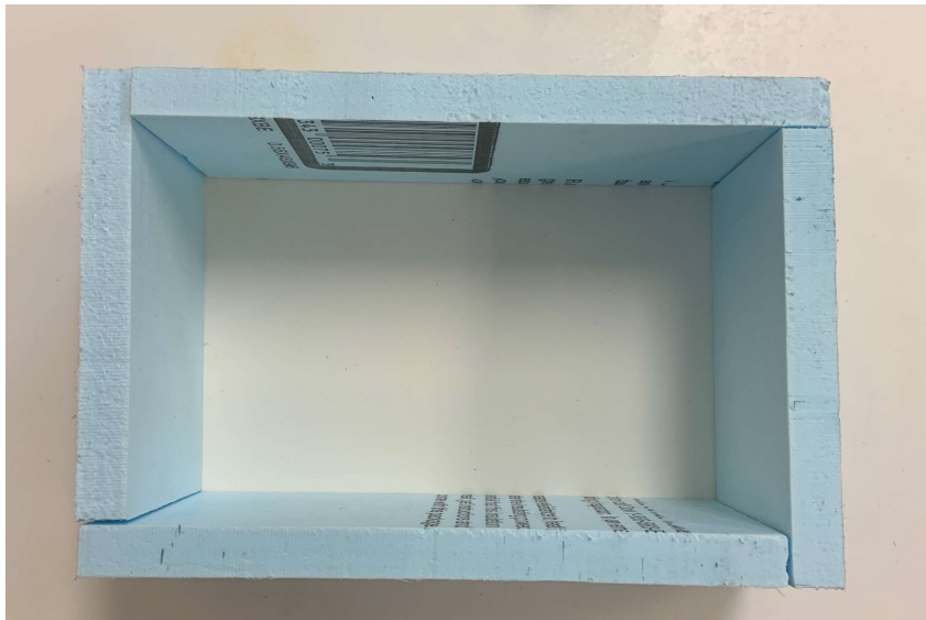
Figure 3: Arrange the walls to ensure they're flush
