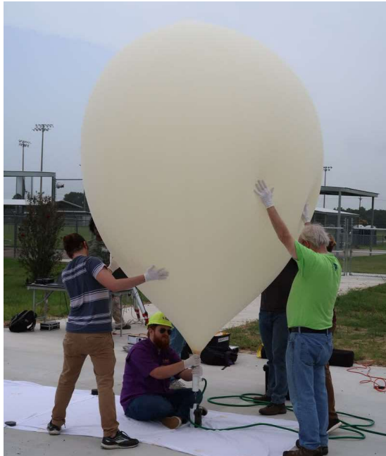
Filling the sounding balloon with helium prior to the ACES61 flight
