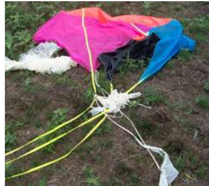
The ACES01 parachute shrouds tangled with balloon remnants
