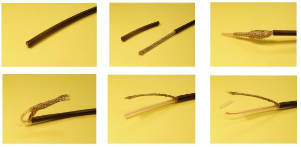
Note that the braided shield is not unraveled, but rather bunched up and separated so that the inner conductor can be pulled through the opening. Both the braid and the inner conductor should be "tinned" before soldering to the board.
