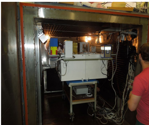
Figure 10: HASP and student payloads in the CSBF BEMCO chamber in preparation for thermal / vacuum testing.
