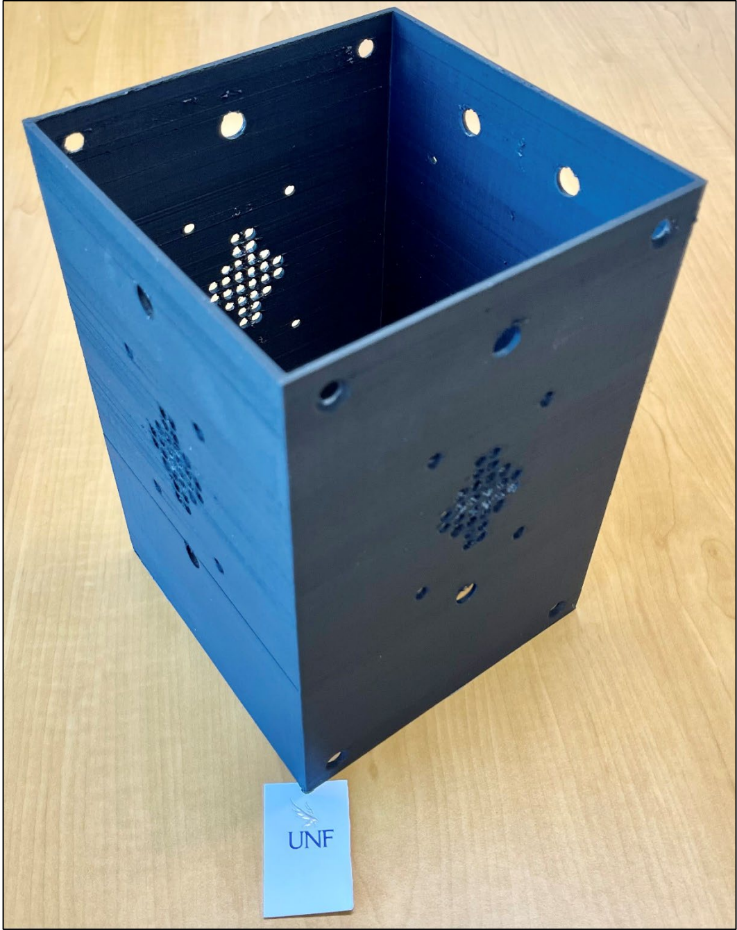
Fig.5 Final 3-D print of the payload body
