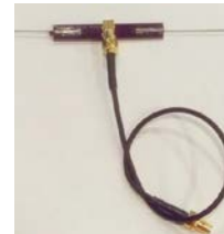
(f) VHF dipole antenna
