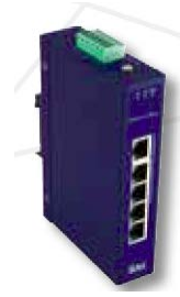
(b) Ethernet switch with case (the case will be removed for the payload)
