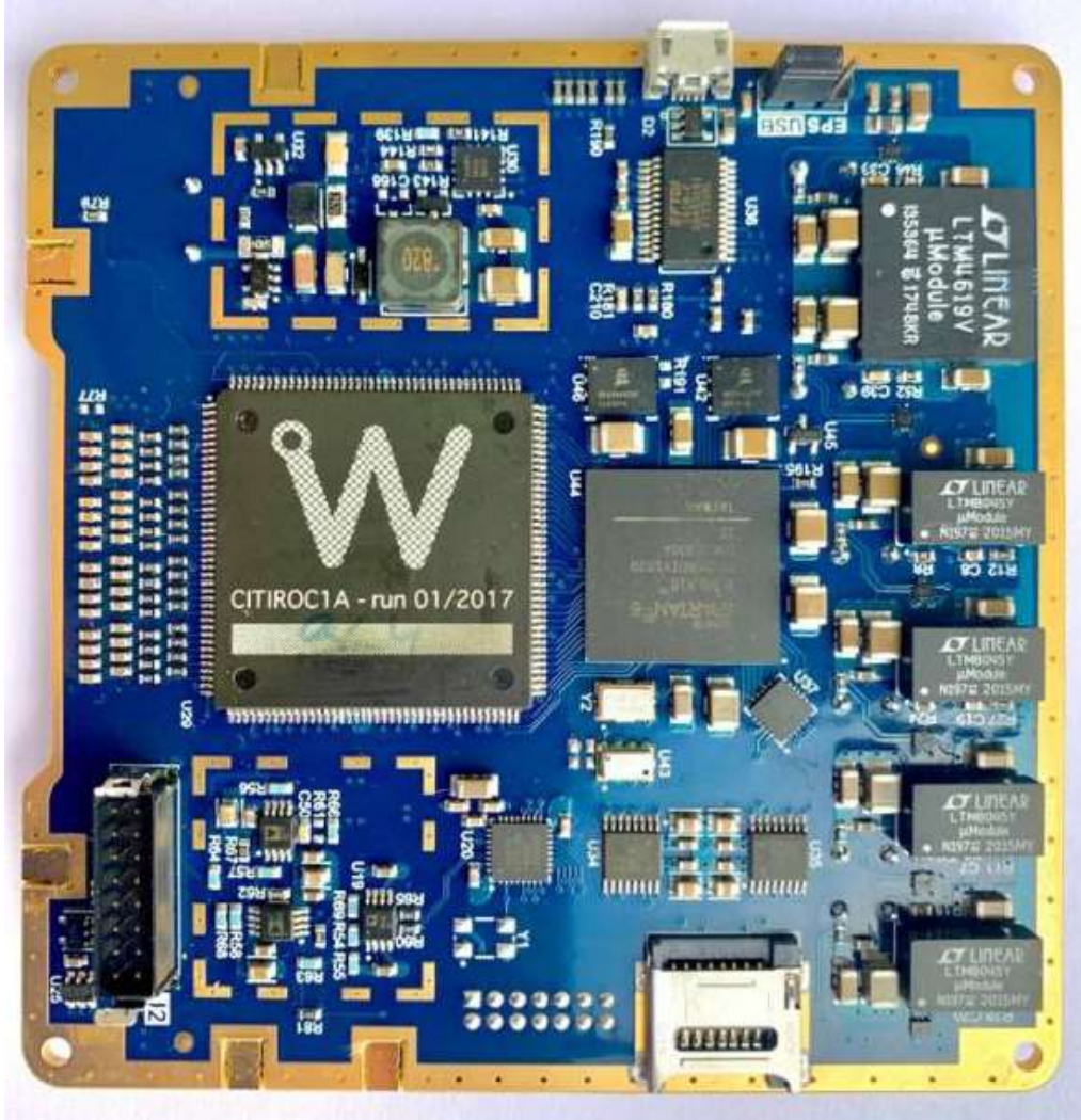
Figure 6 - PCB top of the DAM, fabricated December 2020.
