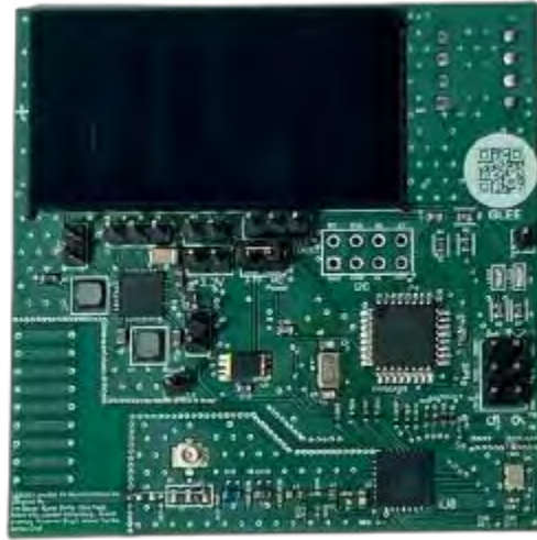
Figure 3: The most recent version of the LunaSat from the GLEE website [2]
