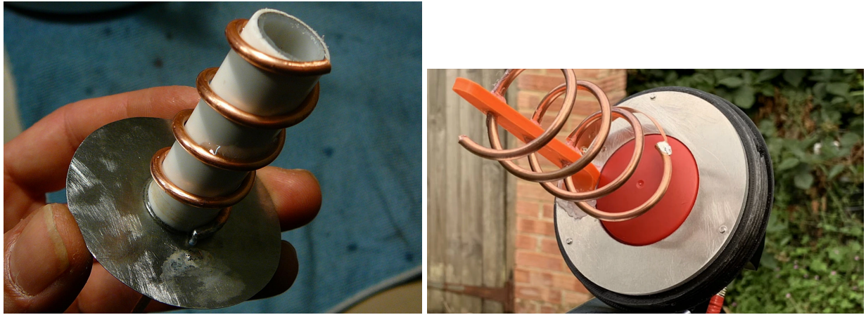
Figure 3: Two methods of supporting the antenna helix. The team will explore both (a) using off-the-shelf plastic tubing [3] and (b) manufacturing a helix holder [4].
