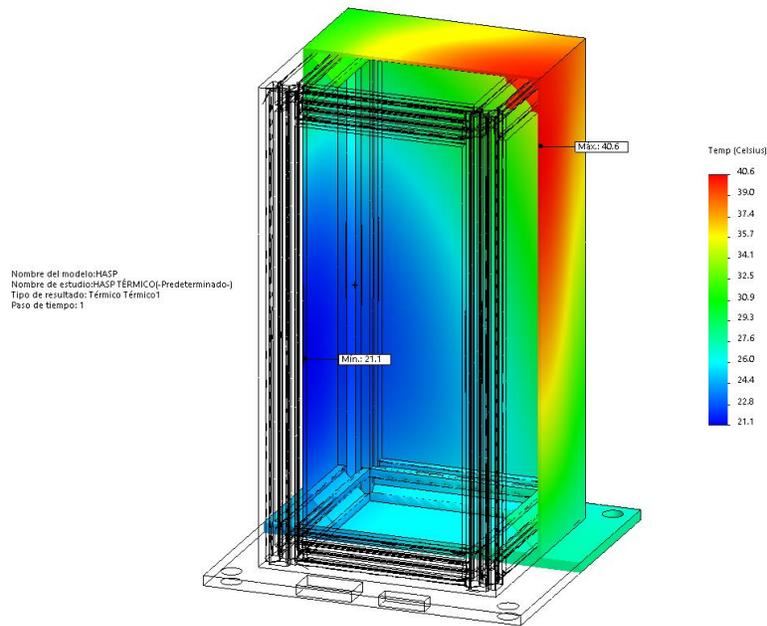
Fig. 33. Internal view of the analysis of the temperature distribution by radiation on the external structure in the SolidWorks® software.
