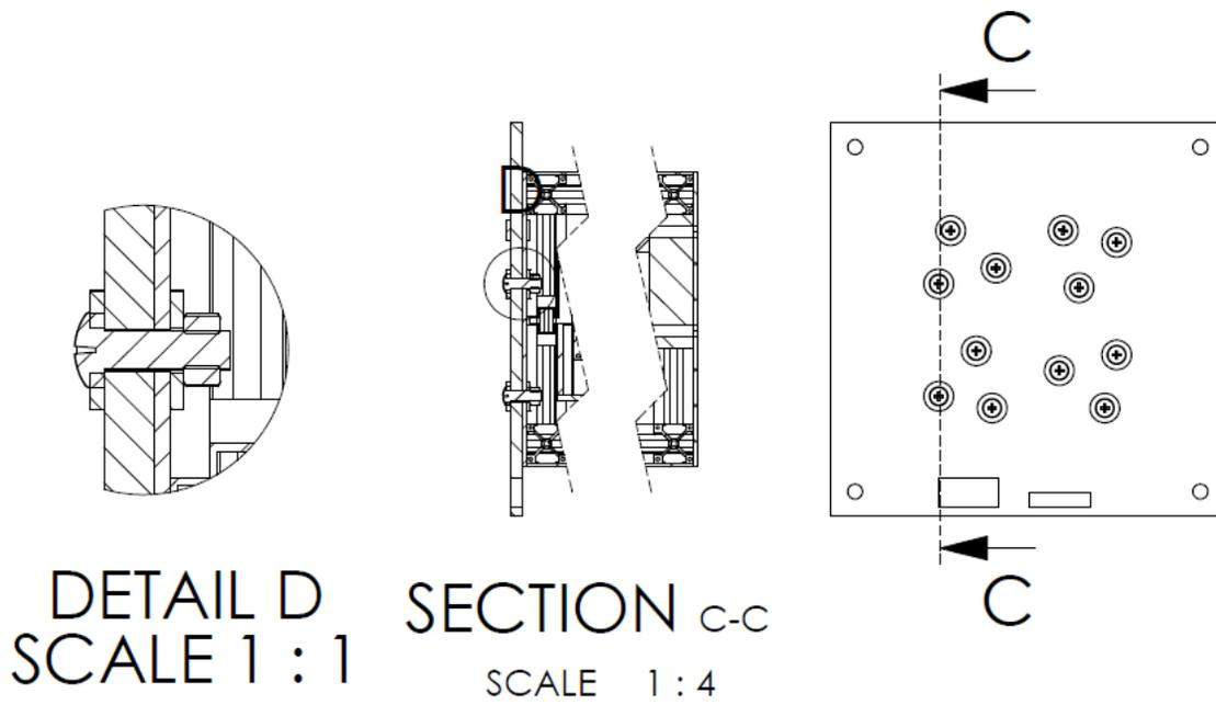
Fig. 12. Fastener cross section.
