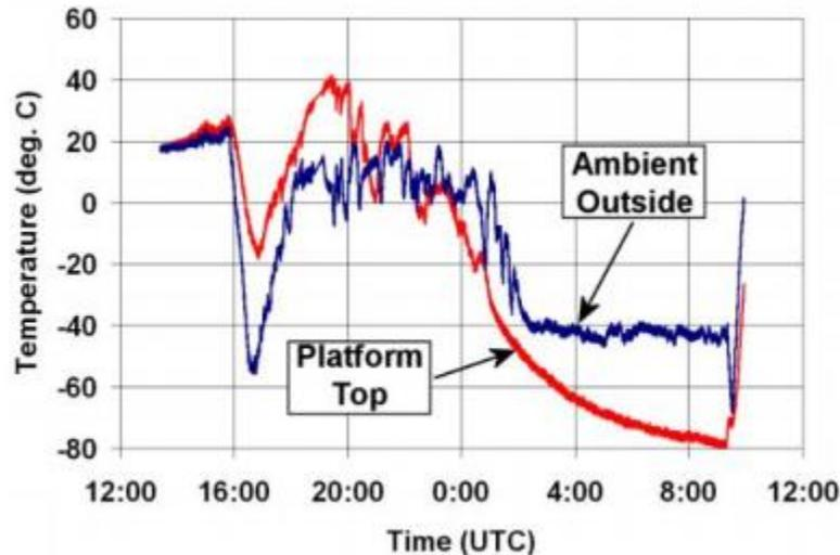
Fig. 31. Typical temperature during flight. (Source: HASP 2021 CFP)
