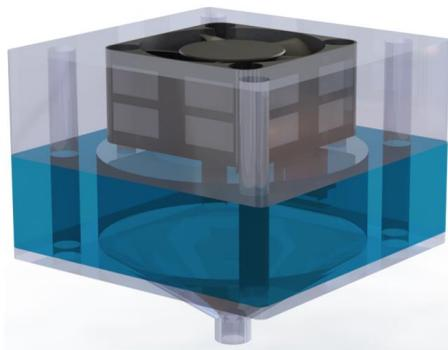
Fig 3. Module for air flow through the cooler with temperature and humidity sensor SHT31.
