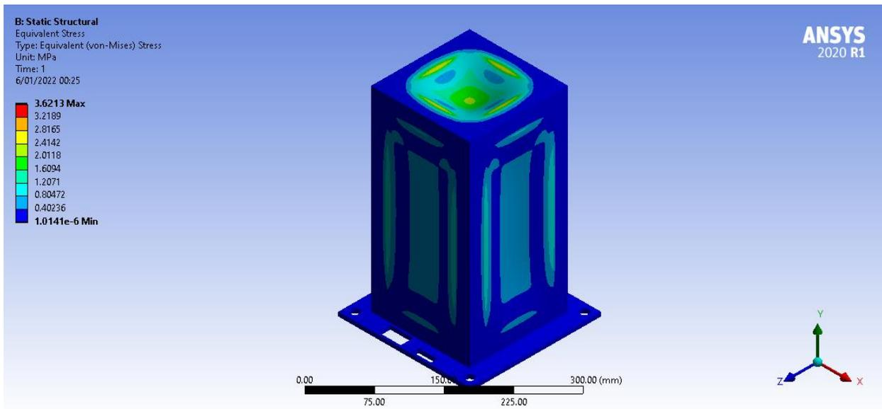
Fig. 9. Stress equivalent to the mechanical structure under a 10 g vertical and 5 g horizontal shock.
