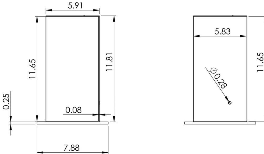
Fig. 41. Payload front view dimensions in inches
