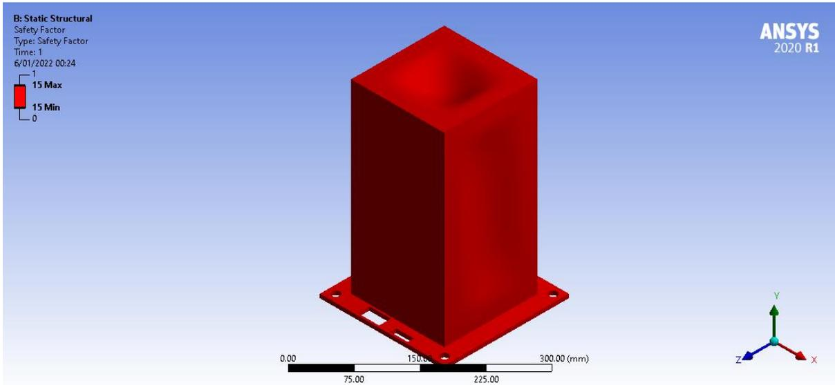
Fig. 10. Safety factor under a 10 g vertical and 5 g horizontal shock.
