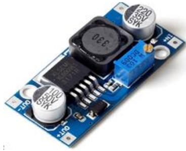
Fig. 23. Step Up XL6009 DC/DC Booster DC/DC Voltage Regulator.
