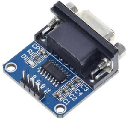
Fig 5. MAX3232 Converter Module - RS232 to TTL
