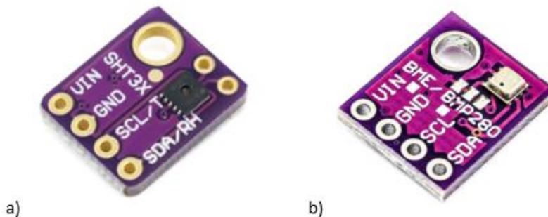
Fig. 15. Humidity and temperature sensors, a) SHT31, b) BME280.
