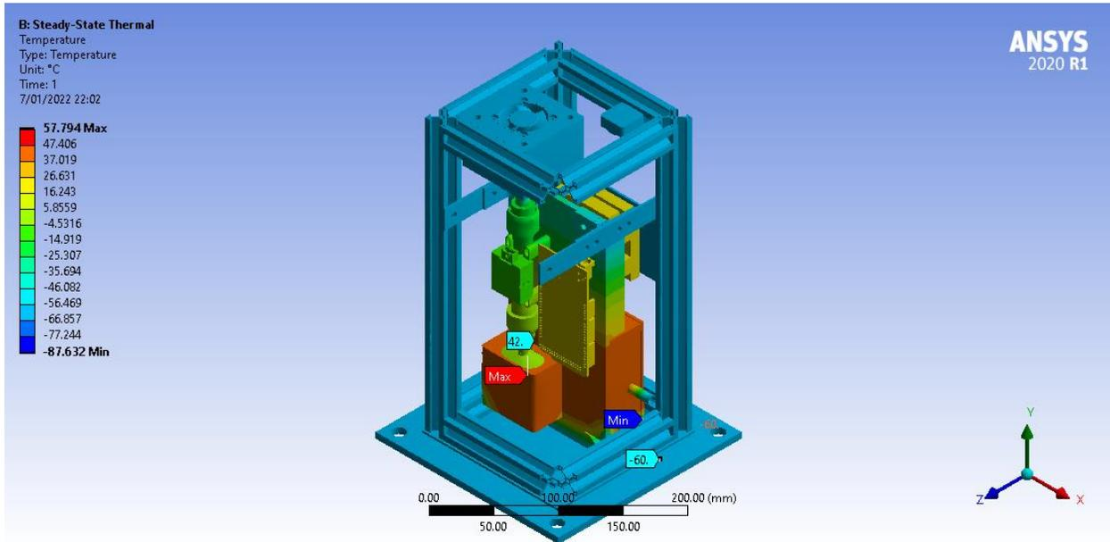
Fig. 35. The internal temperature of the payload considering an external temperature of  $-60^{\circ}\text{C}$  and the heating pad turned on.
