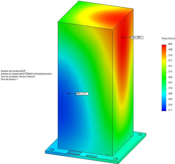
Fig. 32. External view of the analysis of the radiation temperature distribution over the external structure in SolidWorks® software.
