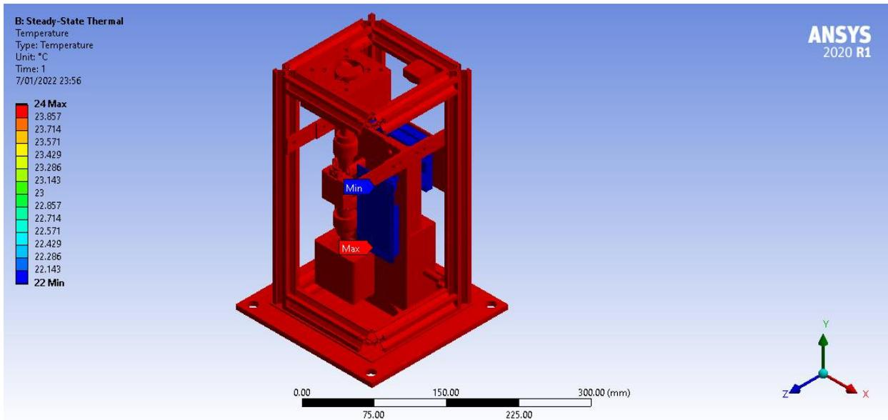
Fig. 34. The internal temperature of the payload considering an external temperature of 24°C and the heating pad turned off.
