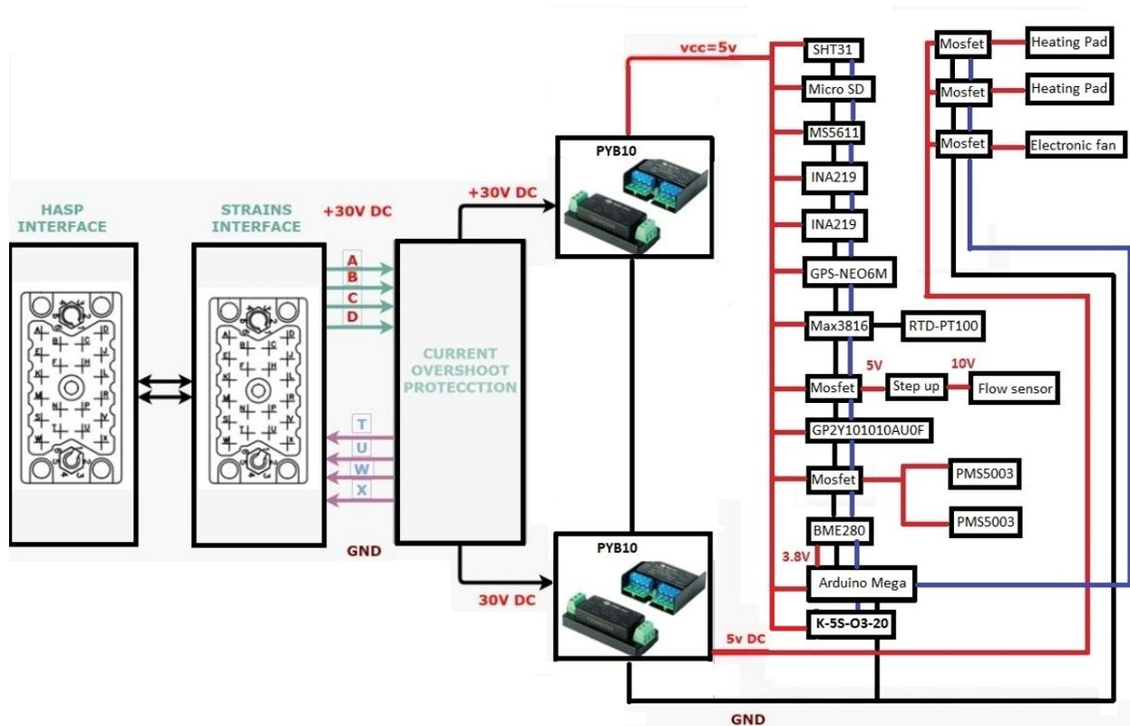
Figure 38. Power Distribution Diagram
