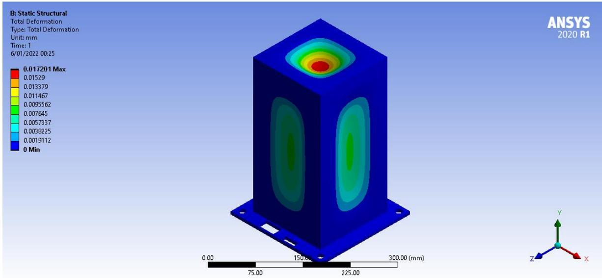
Fig. 8. Total deformation under a 10 g vertical and 5 g horizontal shock.
