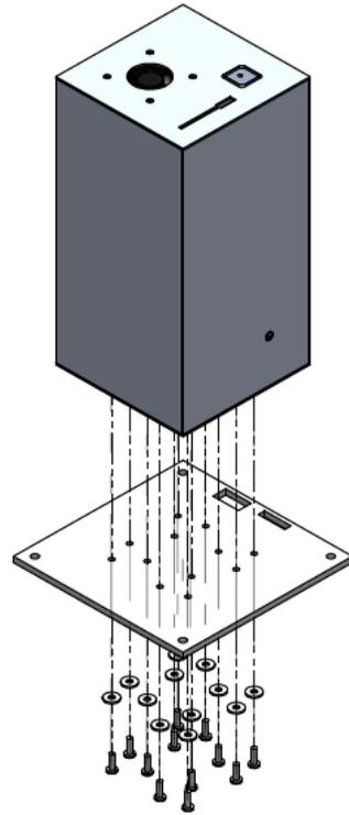
Fig. 11. Payload mounting plate interface.
