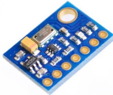
Fig. 16. Pressure and temperature sensor MS5611.
