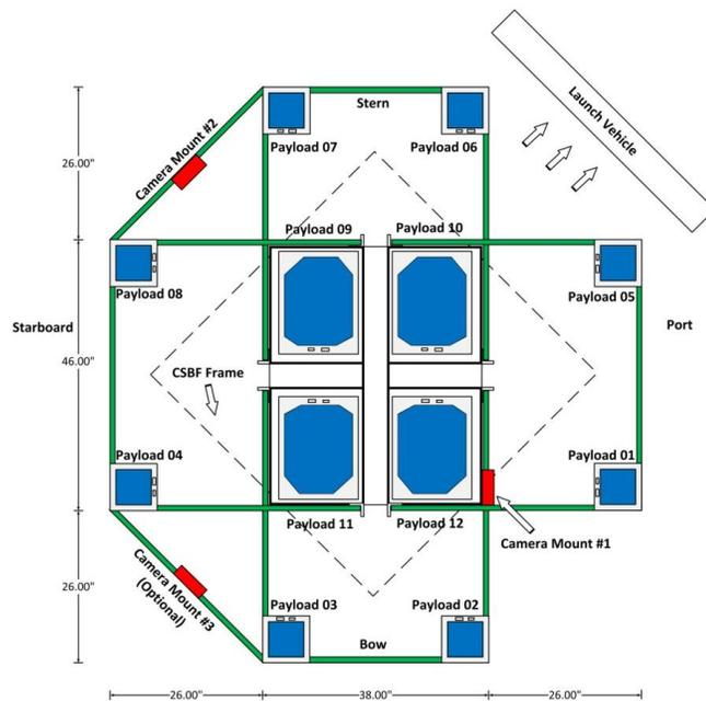
Fig. 37. Top down view of the HASP student payload positions [26]
