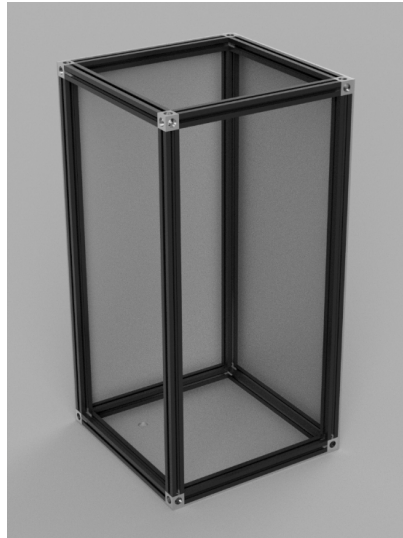
Figure 7: Box design. Dimension: (150x150x300)mm. See figure 19 for dimensional drawing
