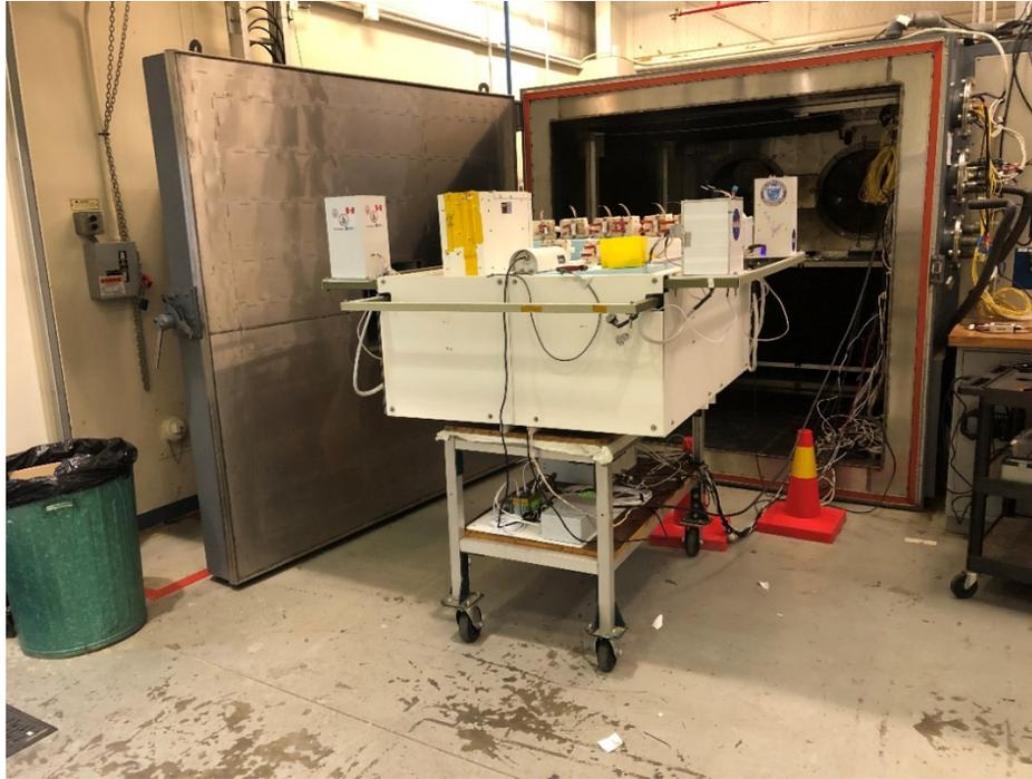
*Figure 23: NASA HASP structure with all payloads experiments of other universities getting ready to go into the chamber for thermal test.*
