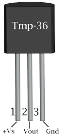
*Figure 18: Temperature Sensors pin-out.*
