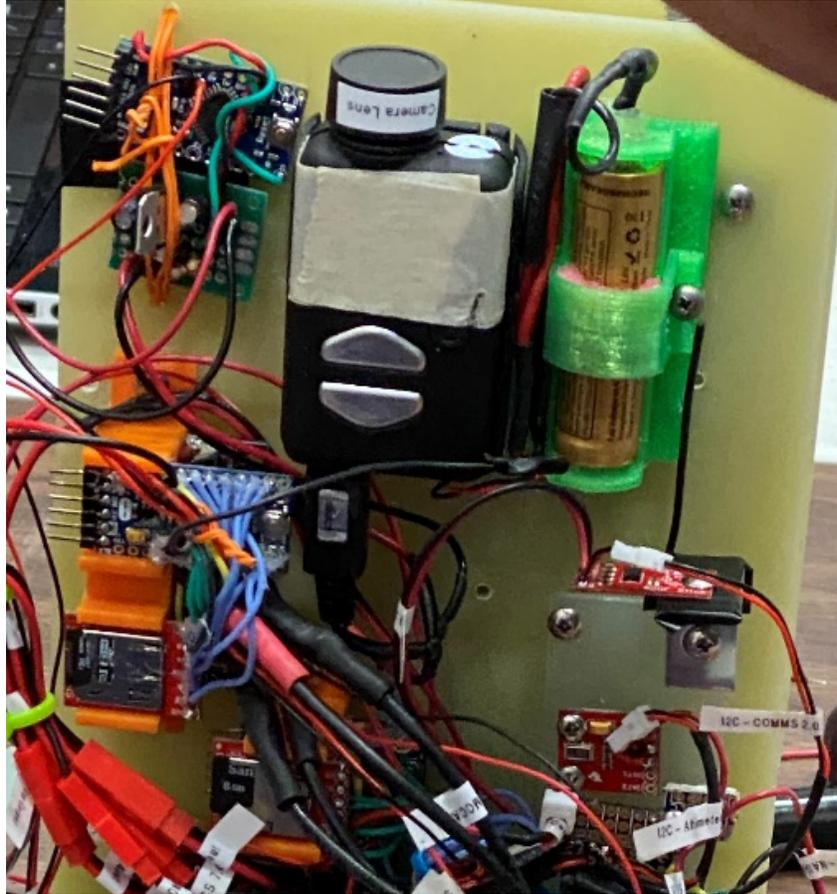
*Figure 13: The mounted mobius camera with power supply next to it.*
