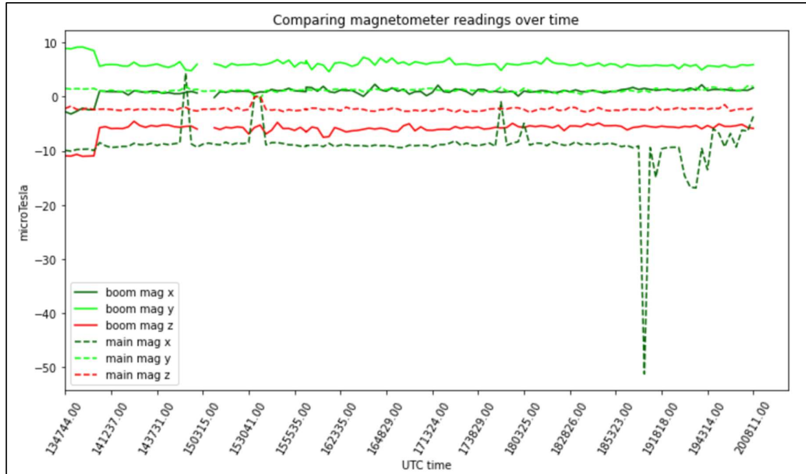
Figure 9: This plot shows the magnetometer readings taken during integration on the first thermal/vacuum test day (7/28/21)
