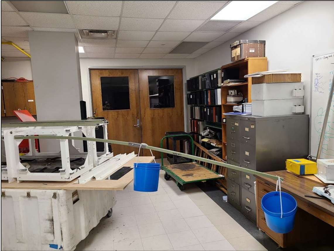
Figure 58: Boom under load during horizontal proof test.
