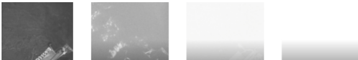
Figure 12. As the OreSat1B payload progresses through flight, images can be seen to degrade in quality over time as the thermal mass saturates and the sensor’s temperature rises
