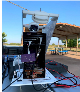
Figure 14. Focus calibration of the OreSat Live Schmidt-Cassegrain telescope before integration in Fort Sumner, NM.
