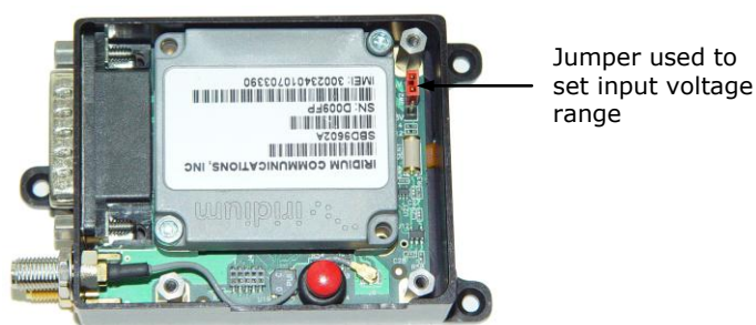
Figure 2. Power Input Setting for the 9602-LP.
