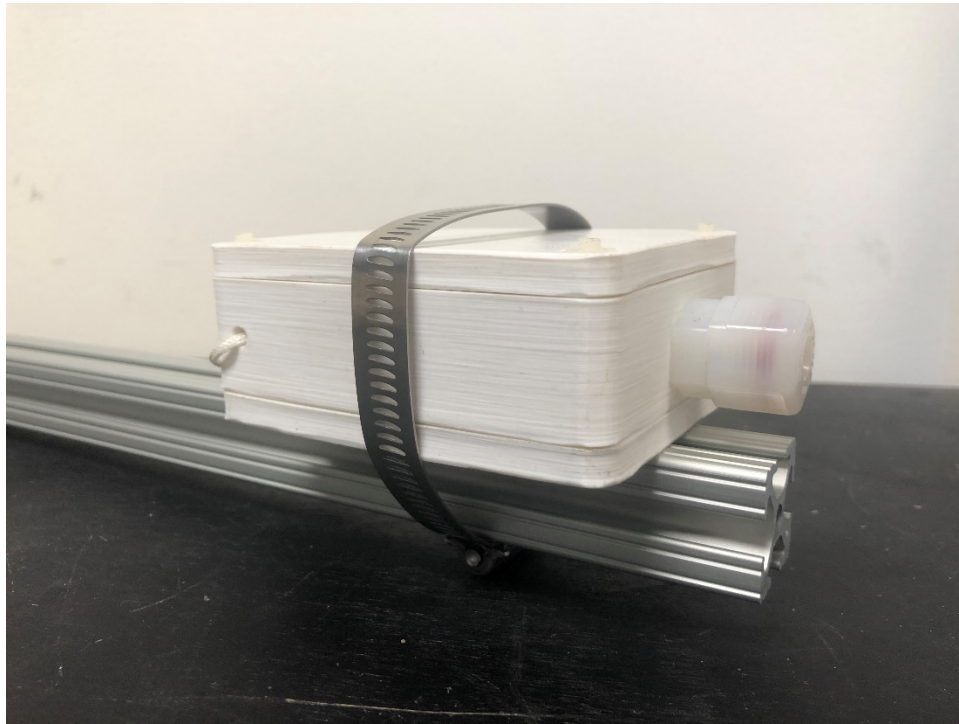
Current cut down hose clamped to 1" aluminum extrusion
