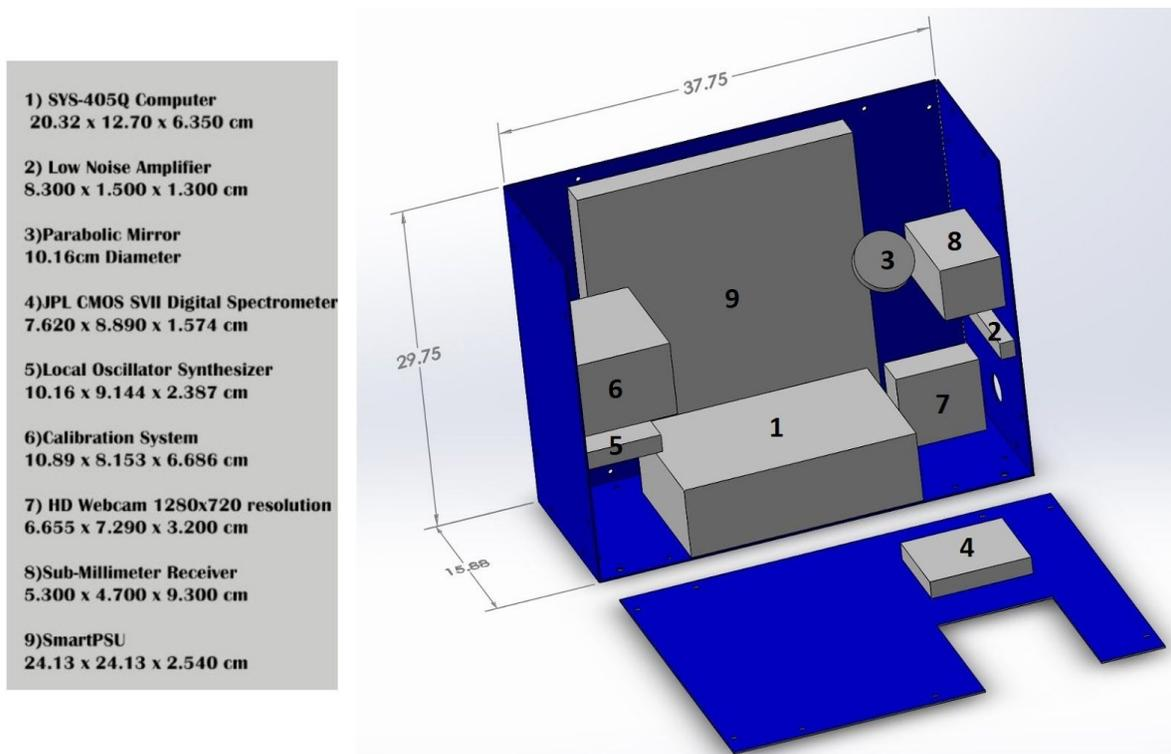
*The Interior of the WWASP Team payload, future iterations of the payload will showcase the step motor, calibration system broken up into its components. etc.*
