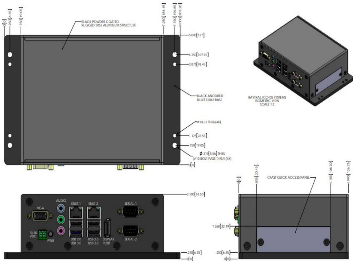
**Housing** – Made of lightweight aluminum, the enclosure provides ample durability without adding unnecessary weight to the system. Its exterior has a black powder coat finish that resists scratches and fingerprints. With its durable exterior and fanless interior, the SYS-405Q is able to survive in industrial applications and reduce field service.
