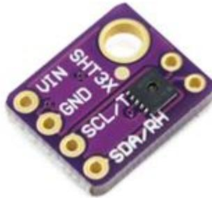
Fig. 11. SHT31 temperature and relative humidity sensor.
