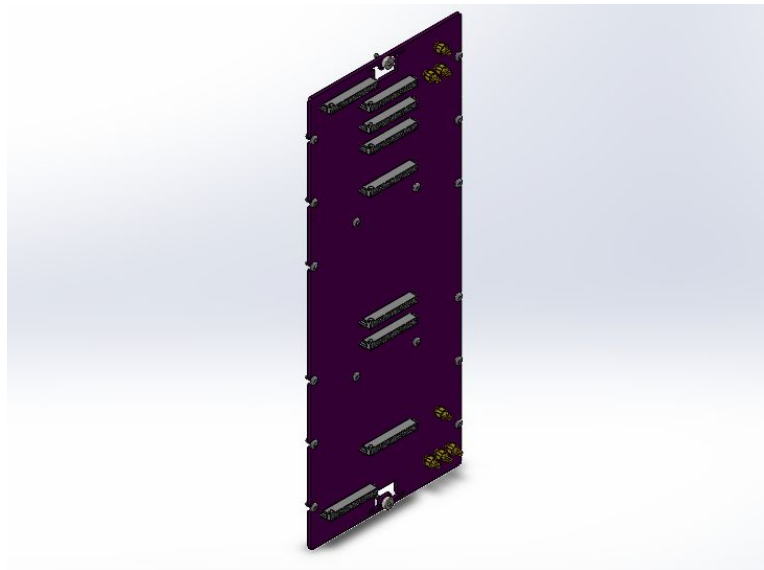
Figure 5. OreSat Backplane Assembly
