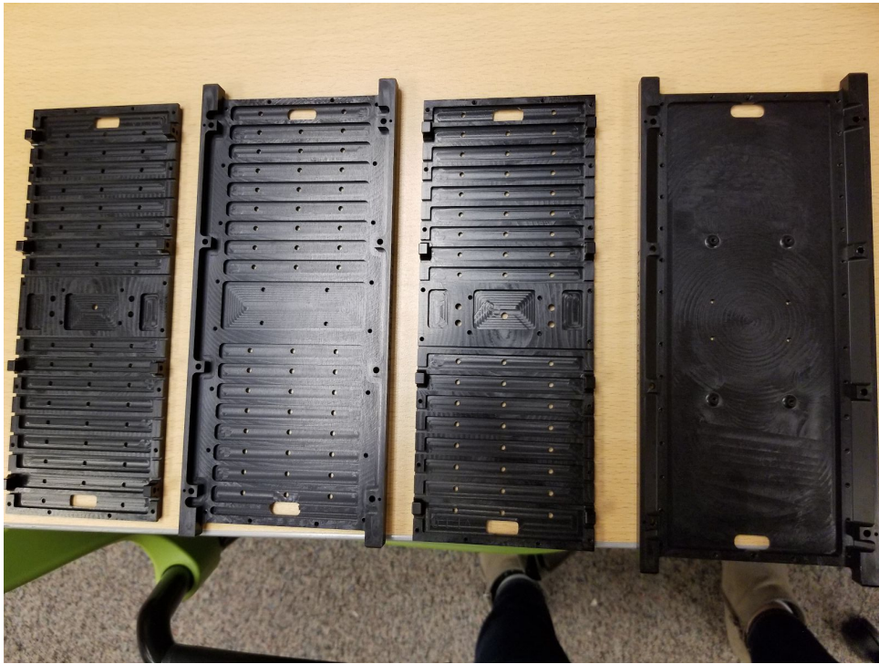
Figure 32. Existing anodized aluminum frames for OreSat
