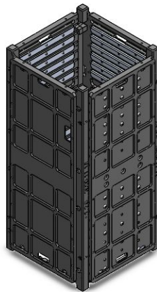
Figure 4. V1.2.0 configuration of the OreSat Frame Assembly
