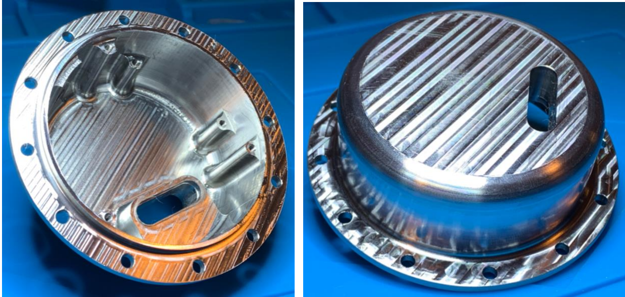
Figure 25: Payload detector vessel base top view (left) and bottom view (right), fabricated November 2020.
