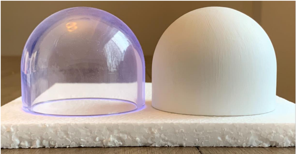
Figure 27: Scintillators manufactured in December 2020. Scintillators were manufactured with (right) and without (left) polishing and a reflective paint coating to determine which will show better performance.
