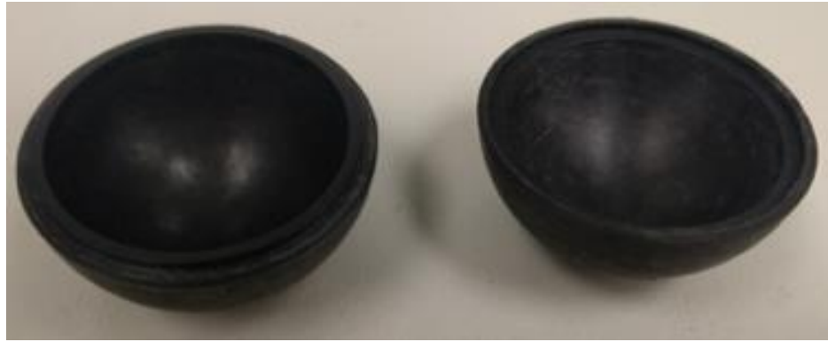
Figure 20: Undercut (left) and overcut (right) hemispheres to make the TE sphere, fabricated in March 2019.
