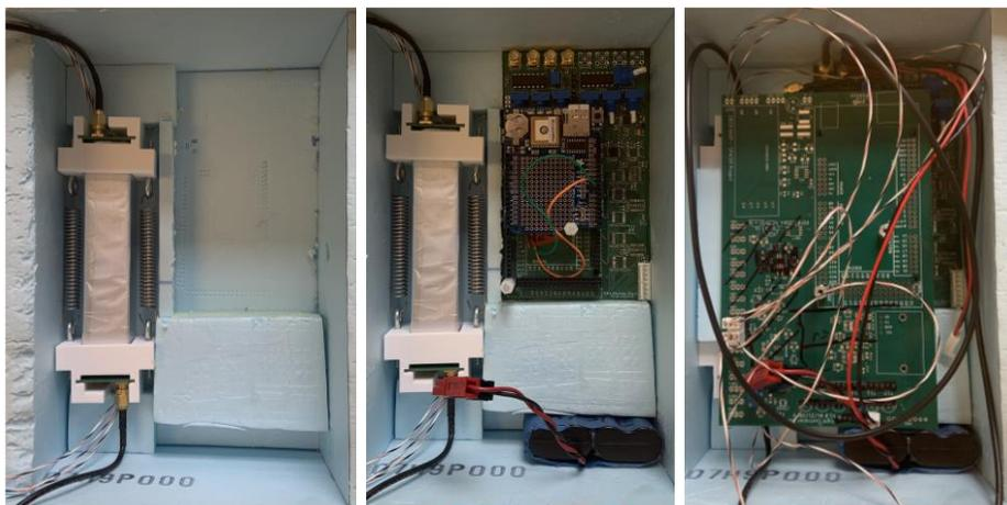
Figure 10: Illustration of the assembly of the scaled-down SPACER payload flown on June 6<sup>th</sup>, 2019
