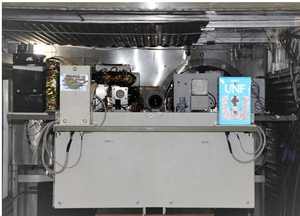
Fig. 19 (b) Inner view of a thermal vacuum test chamber shows stray light, light bulb, and radiation heaters in the chamber.
