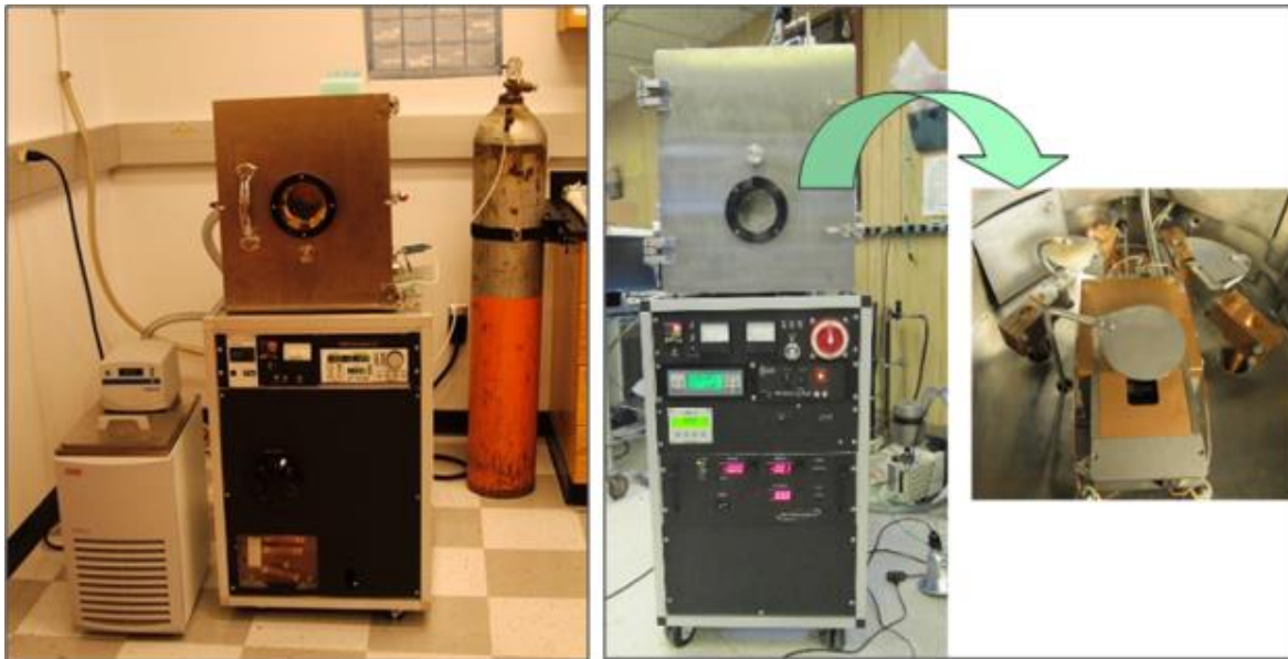
Fig. 3 (a) Thermal vacuum deposition system and (b) electron beam deposition system.
