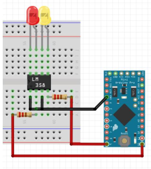
Figure 5: Mobius camera wiring diagram. The LEDs represent camera buttons.
