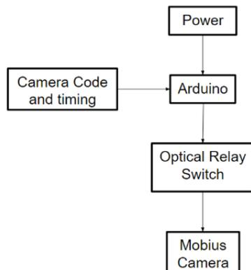
*Figure 4: Mobius camera block diagram.*
