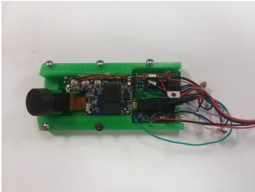
Figure 6: Top down view of Mobius camera.
