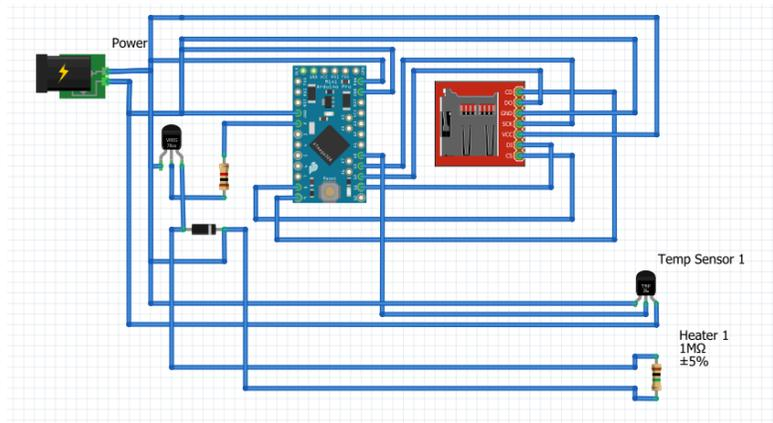
Figure 11: TMS circuit schematic for one heater and sensor.
