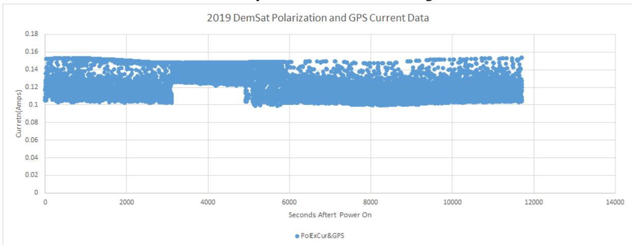
Figure 37: Polarization and GPS current draw.
