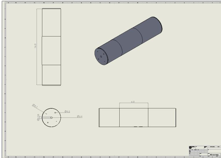
*Figure 18: Outer structure drawing for DemoSat.*
