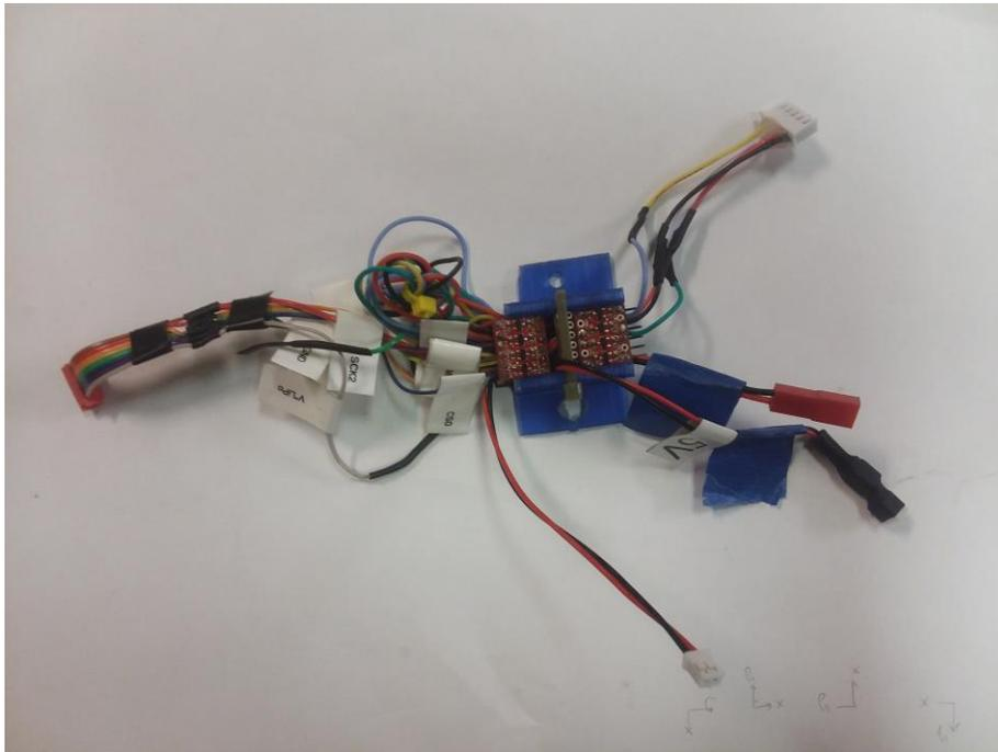
*Figure 14: Comms Wiring*
