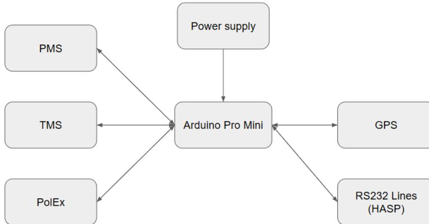
*Figure 13: Communication system Block Diagram*
