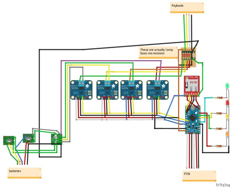
Figure 8: PMS circuit diagram
