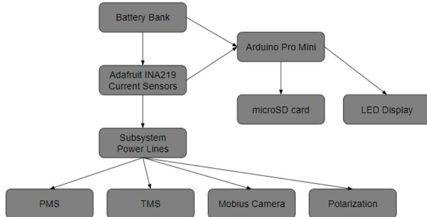
Figure 7: Power management system block diagram.
