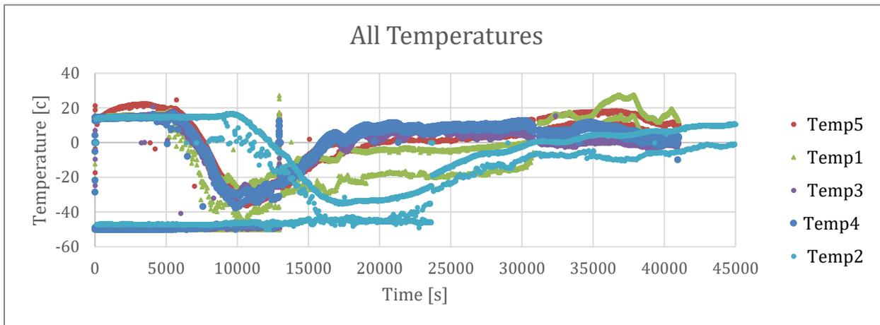
Figure 27: Temperature over time of flight for all subsystems.
