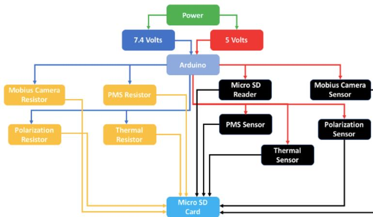
Figure 10: Thermal system block diagram.
