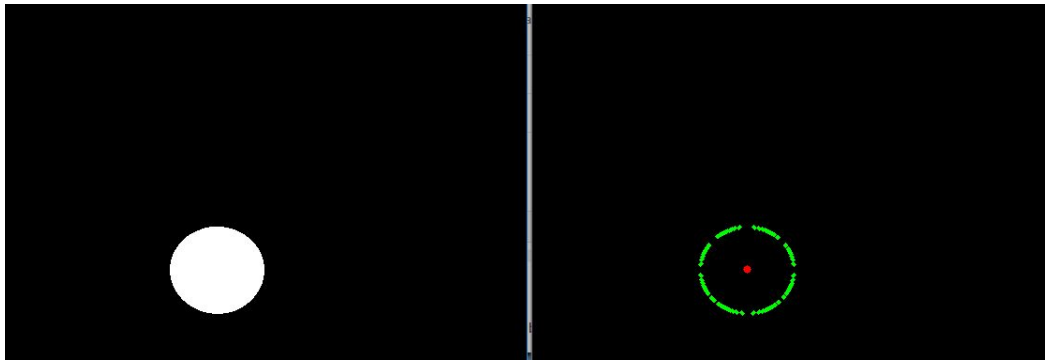
Figure 4.3.2.6.a: Wrapping Contour Around the Detected Object
