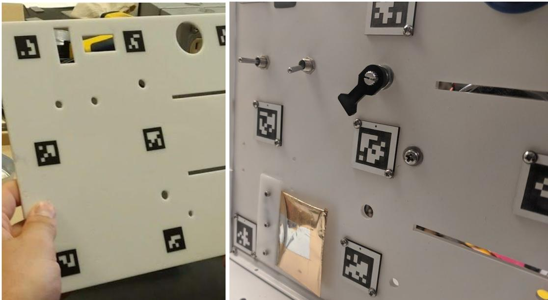
*A set of vinyl-cut fiducials, from the AprilTag family 16h5 (left) and laser-etched 2-ply acrylic fiducials from AprilTag family 36h11 (right), both on laser-cut acrylic plates.*
