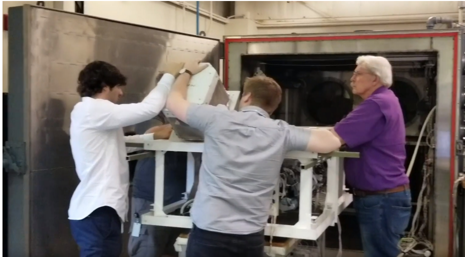
Figure 44: The team installing the payload on the HASP platform prior to TVAC testing
