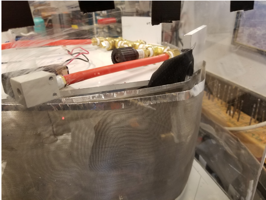
Figure 33: The location of the Ripstop after rupture
